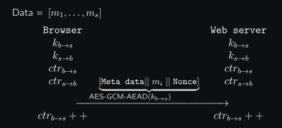
Meta data includes: record on the phase (1 or 2), TLS Version, len(c)Counters ctr are used to prevent replay attacks OpenSSL provides interfaces to GCM, CCM AEs via EVP
